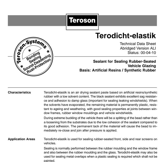
**Technical Data** Colours: black Odour: smells of petrol Consistency: paste Density: ca. 1.5 g/cm<sup>3</sup> Solids: ca. 87 % Sag resistance: good In service temperature range: -30°C to 80°C Short exposure (up to 1 h): 100°C
